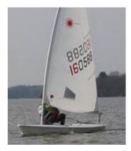
The **Laser** is a widely used class of single-handed, one-design sailing dinghies using a common hull design with three interchangeable rigs of different sail areas, appropriate to a given combination of wind strength and crew weight. Bruce Kirby designed the Laser in 1970 with an emphasis on simplicity and performance.
